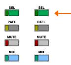
**To assign a Single Strip** Touch the Single Assignment button. Press the SEL key on the strip you want to assign. Use the drop down menu to select the Channel Type you wish to assign. Touch the Channel Number box to highlight it and use the screen encoder to scroll to the number required. Touch Apply to accept the change.
